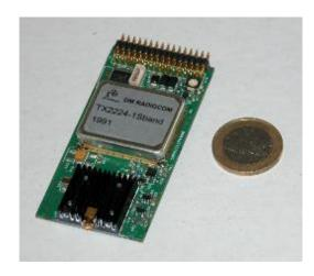
Data rate PCM/FM: 1 to 14 Mbps. Signal interfaces: PCM/FM input 1V peak to peak no base band filter 50 ohms.
